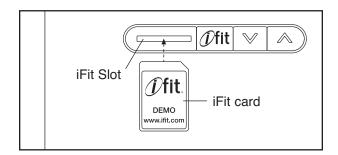
Next, select the desired workout on the iFit card by pressing the increase and decrease buttons next to the iFit slot.
